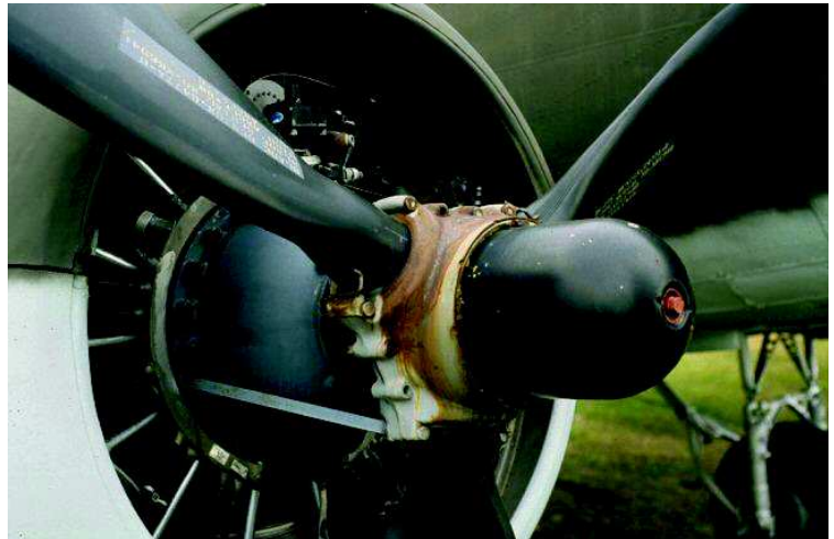
The curved tubes at the base of the propeller blades delivered anti-icing fluid (isopropyl alcohol) to the grooved edges. (Douglas C 47...ou DC 3)
