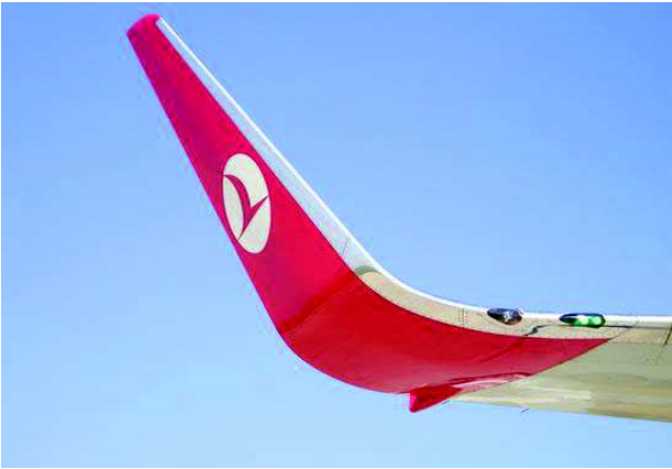
Winglet du type Boeing ( Blended Winglet )
