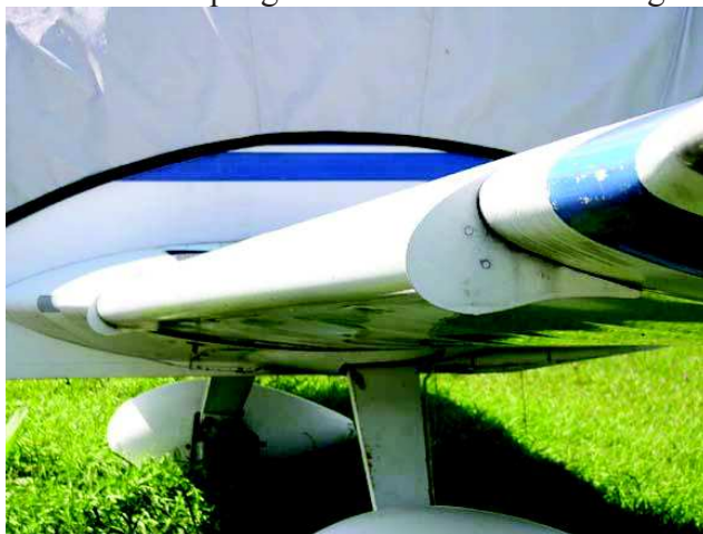
A drooped leading edge cuff installed on an American Aviation AA-1 Yankee as part of a NASA experiment
